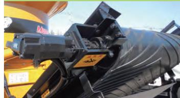
You can perform crushing operations with peace of mind, as it effectively removes nails and other materials that may be mixed in with construction waste, ensuring their safe disposal.
