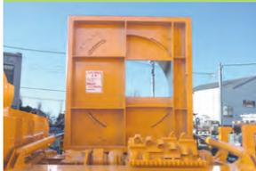
The input hopper table can be opened and closed at a 90° angle, allowing for maintenance tasks such as screen or cutter blade replacement and cleaning.
