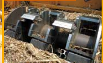
Knife type cutter drum
